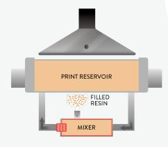
CONTINOUS: Resin is circulated throughout the printing process KINETIC: Mixing energy is tuned for each material
