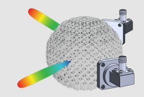
Dielectric GRIN lenses can be used to augment performance of standard gain horn antennas. Mounting a lens to a horn can increase directivity and gain, collimate the wavefront, or convert a diverging wavefront into a converging, spot focusing signal. Customers often pair 3D printed lenses with horn antennas when high gain is required in minimum space, or to rapidly modify the performance characteristics of existing equipment.
