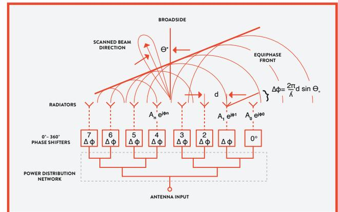
**Figure 4:** Linear phased antenna array during a scanning operation.
