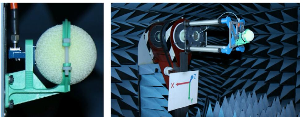
**Figure 15:** Left - The 3D printed GRIN lens mounted to the fixture in front of the open ended waveguide feed source. Right - The mounted lens affixed to the test rig in the anechoic test range.
