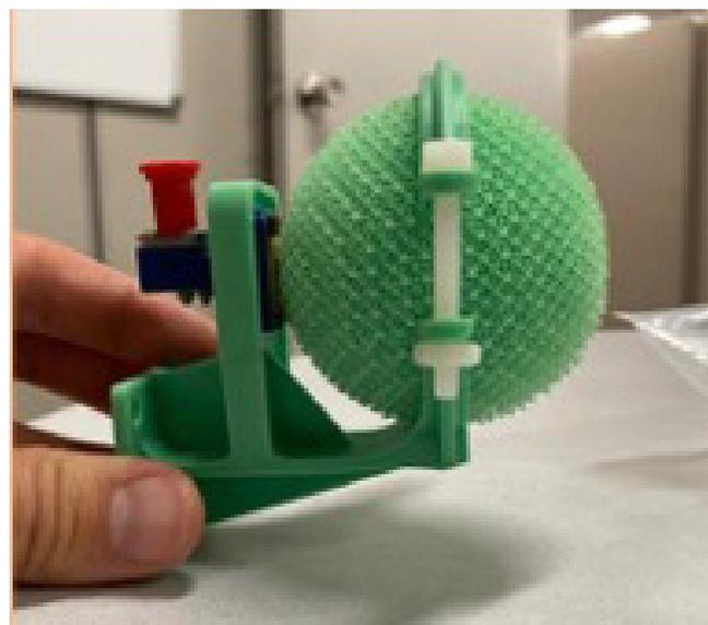
**Figure 17:** GRIN Luneburg lens built using conventional, commercially available photopolymer resin.
