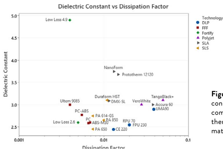
**Figure 10:** This chart plots the dielectric constant and loss tangent of several commercially available commodity thermoplastic and photopolymer 3D printing materials.
