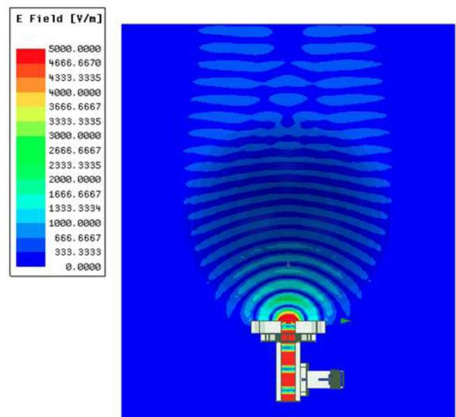
**Figure 12:** Lens design modeled in Ansys HFSS showing the electric field being focused by the GRIN structure.
