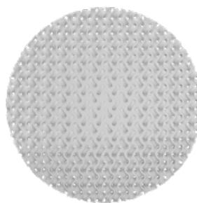
**Figure 13:** This device cross-section shows how the volume fraction of material reduces radially from the center of the sphere to the surface.
