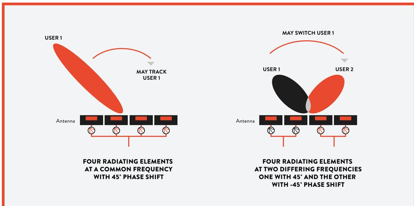
Figure 2: A beamsteering antenna
