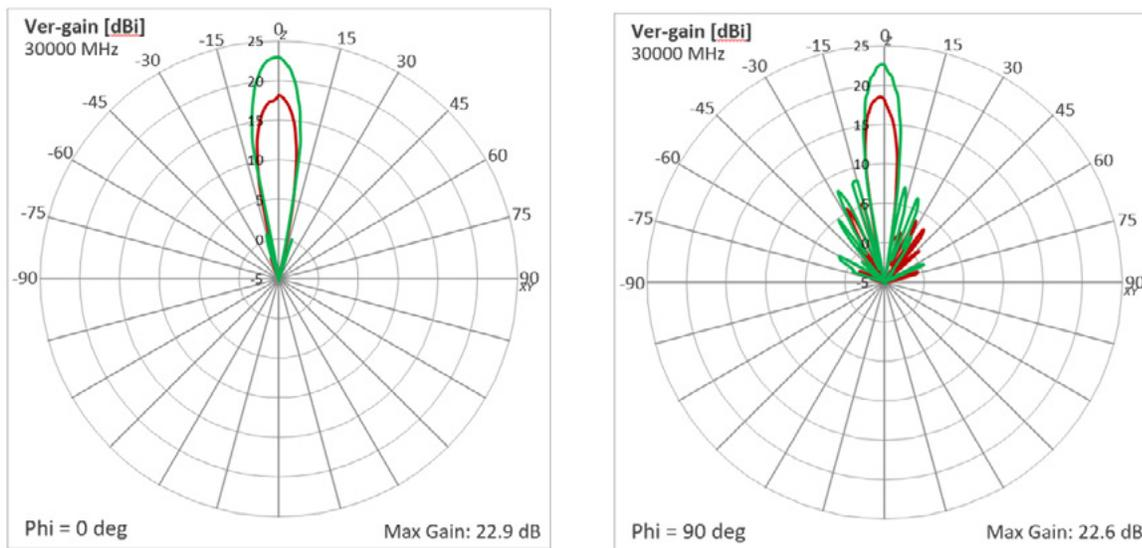
**Figure 18:** 30 GHz test results for the two lenses. In both charts, the green curve is the Rogers and Fortify printed lens, where the red curve is the comparative lens printed with commercially available photopolymer. Left chart -  $\Phi = 0$ . Right chart -  $\Phi = 90$ .
