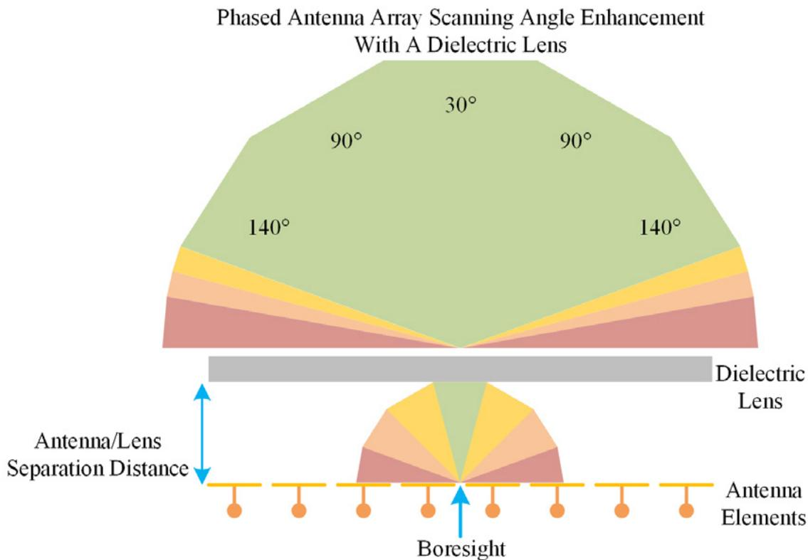
**Figure 7:** A phased array antenna augmented with a dielectric lens for enhanced scanning angle.
