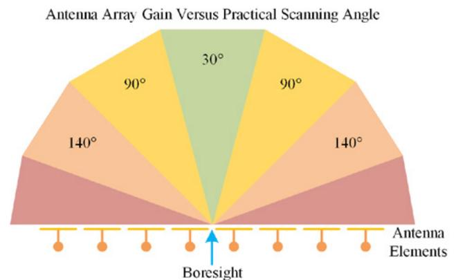
**Figure 5:** A depiction of a linear phased array’s gain performance at various angles away from the boresight with green being the highest and red being the lowest.
