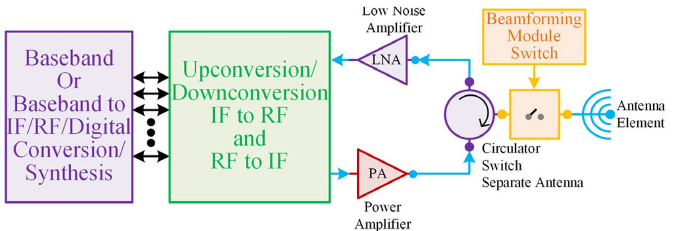
**Figure 9:** Example dielectric lens switched antenna array signal chain for a single element.
