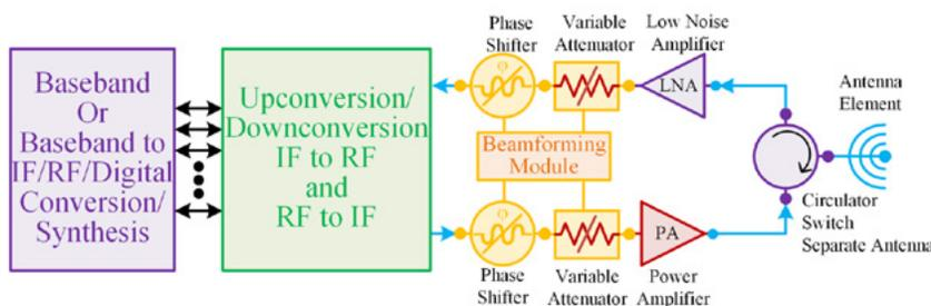
**Figure 6:** A simplified RF frontend (RFFE) for a phased array antenna element that is directly driven.
