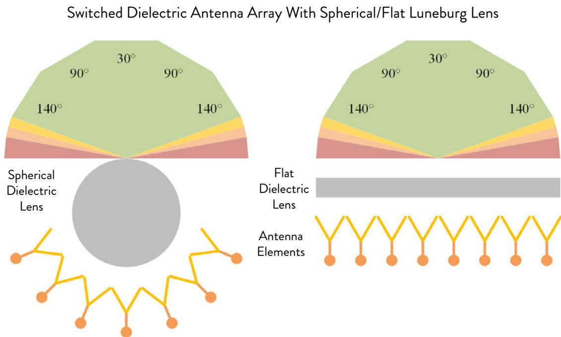
**Figure 8:** (left) A spherical dielectric lens with an array of feed antennas that can be operated as a switched antenna array with wide scanning angle. (right) A flat panel antenna array made using switched antenna feeds and a sophisticated dielectric lens.
