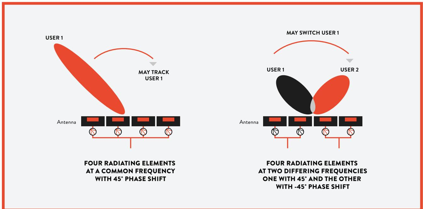
Figure 2: A beamsteering antenna
