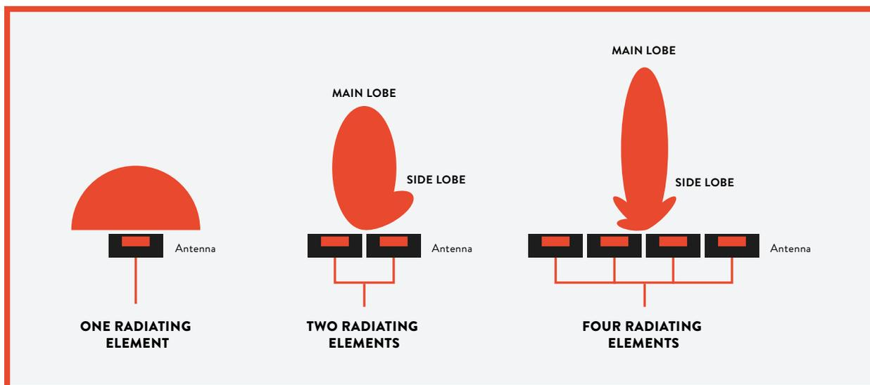
**Figure 1:** A depiction of beamforming antenna pattern behavior as a function of linear antenna elements
