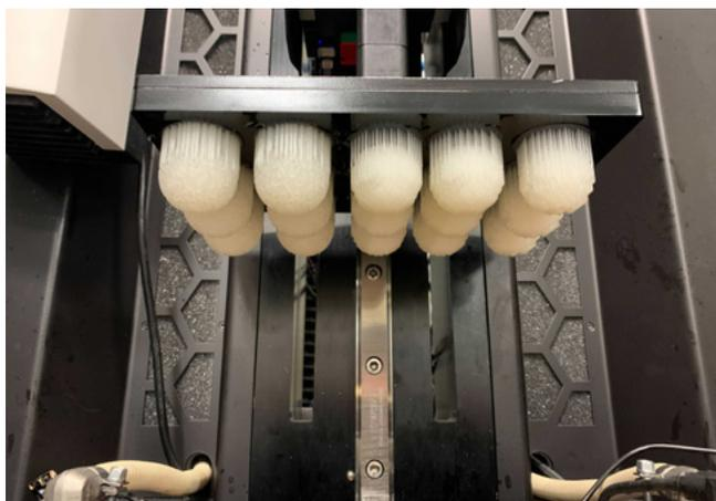
**Figure 20:** Image of a Luneburg-style lens printed on a Fortify Flux Core printer.
