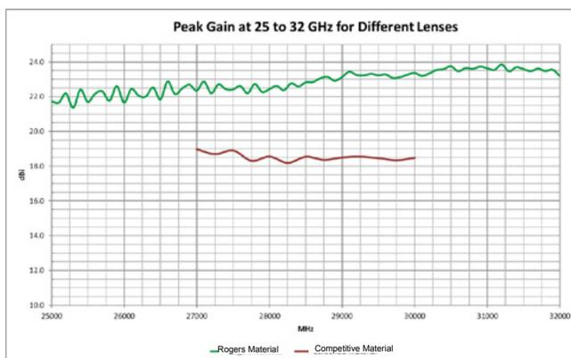
**Figure 19:** This chart shows the max axis gain and peak gain from any direction as a function of frequency. As frequency increases the gain increases, as the aperture size is larger relative to the wavelength. The green curve represents the Rogers and Fortify printed lens, where the red curve represents the comparative lens printed with commercially available photopolymer.
