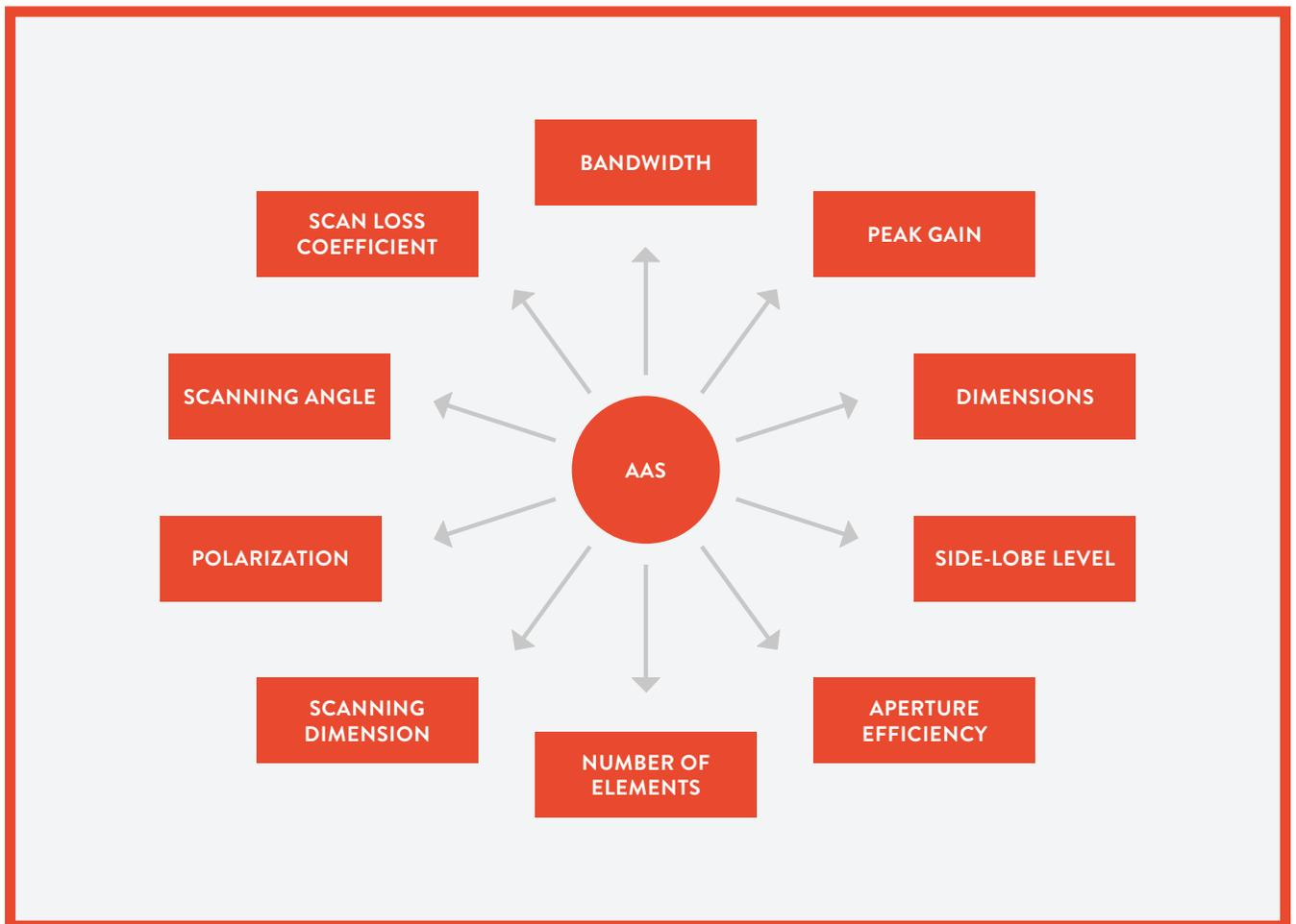
**Figure 3:** The main figures-of-merit (FOM) for AAS
