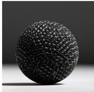
3D-printed Luneburg-style gradient dielectric lens fabricated with the Low Loss 2.8 dielectric polymer.
