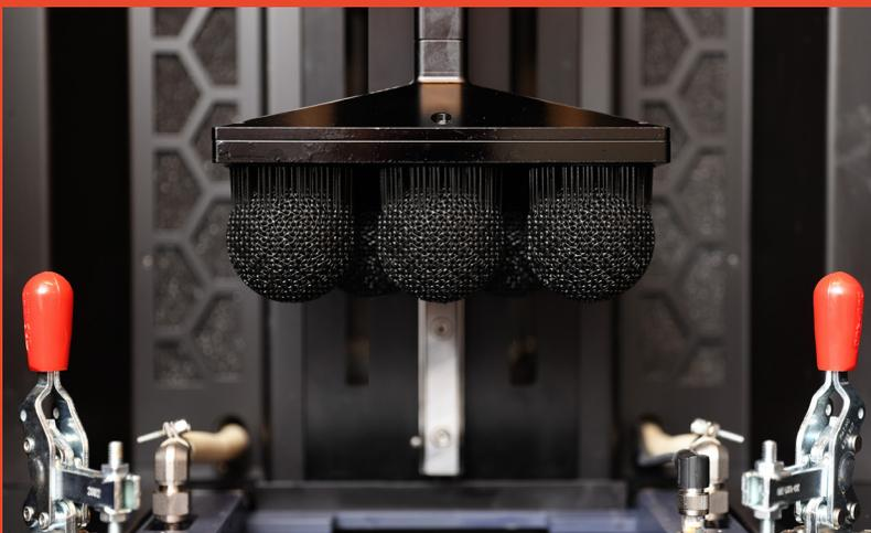
Leveraging lattice-based design, the Fortify platform can print functionally graded architectures - generating monolithic components with smooth gradients of effective permittivity perfect for **GRIN** applications. These low loss materials are an excellent choice for printing **lenses**, wave-guides, connectors, and substrates.
