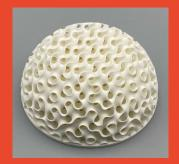
A 3D printed ceramic graded refractive index (GRIN) lens printed on the FLUX CORE pinter with High Purity Alumina (99.8%) (HP-A 99.8) resin.
