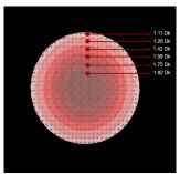
3D-printed Luneburg-style gradient dielectric lens fabricated with the Low Loss 2.8 dielectric polymer.
