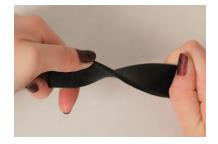
Fortify's ESD-Elastomer is an ideal material for printing high resolution and bespoke PCB boots to provide sensitive components with mechanical and electrical protection
