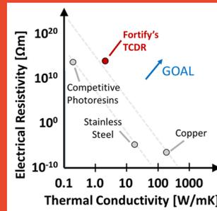
TCDR offers exciting levels of thermal conductivity while maintaining very high electrical resistivities required in many applications.
