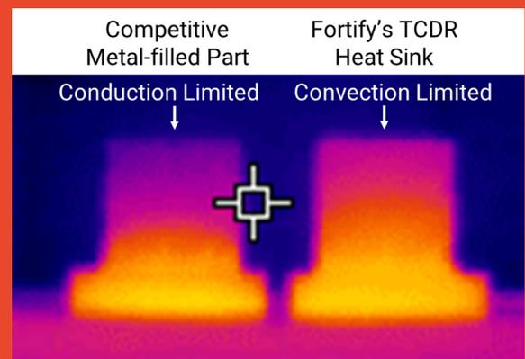
A forward-looking infrared (FLIR) camera takes an in-situ image of a high resolution TCDR heat sink relative to a competitive comparable metal-filled part. Within the metal-filled part, heat builds up near the lower hot surface due to a lower thermal conductivity. Instead, the heat sink made from Fortify's TCDR effectively moves heat through the heat sink and shows signs of being convection limited suggesting further increases in thermal conductivity wouldn't bring much value.
